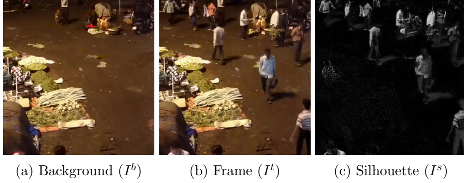
Figure 3.1: An example of background subtraction. The Left image is the computed background ( I^b ), the image in the center is an actual frame ( I^t ), and the right image is the computed silhouette ( I^s ). Clearly, in this case, silhouette detects pedestrians along with their shadows.
